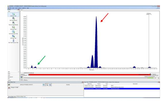
**Figure 2.** Comparison of H2O to H2 partial pressure [a.u.] on a linear scale after 12-hour cryo-cycle and subsequent cooling of system to LN2. The red arrow points to the H2O peak and the green arrow to molecular hydrogen.
