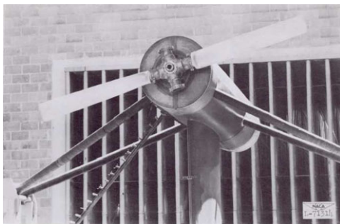
Figure 11. Installed NACA propeller on the Langley dynamometer for the experimental study of Allis and Swihart [34].
