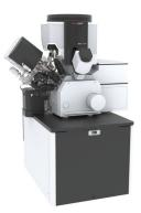
The Helios 5 Laser PFIB enables high-quality subsurface and 3D characterization at millimeter scale with nanometer resolution. It provides large-volume 3D analysis, gallium-free sample preparation, and precise micromachining. With an integrated femtosecond laser, it offers fast material removal rates while maintaining high cut-face quality. The Helios 5 Laser PFIB combines (a) the Elstar SEM column, for ultra-high-
