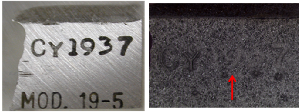
Figure 1. Left - serial number after initial grinding step. Right – serial number following after ‘9’ has been ground away, shown in etch relief (arrow).
