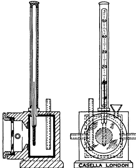
Fig. 1. Side and front view of dew-point apparatus.
