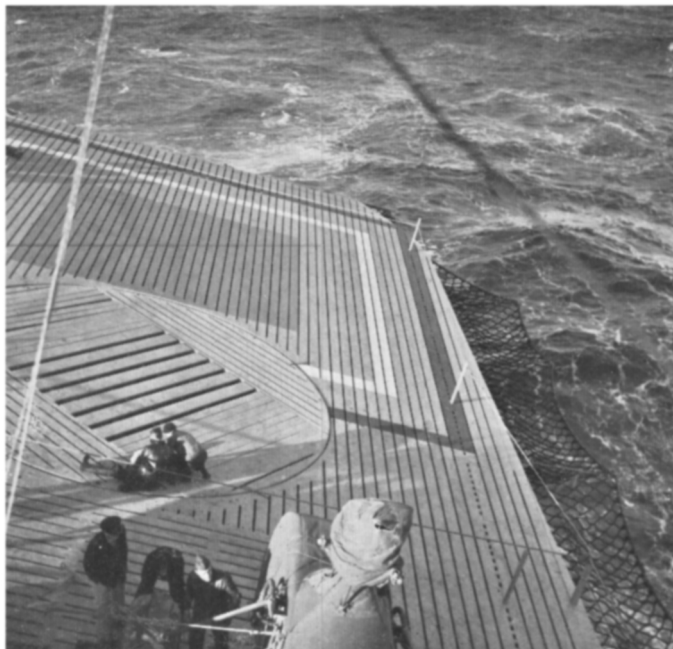
Fig. 10. A typical example of an unstable platform. To facilitate shipboard operation, positive anchorage of the helicopter to the deck is essential.
