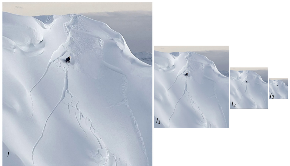
Figure 3. Gaussian pyramid, where subsequent images are weighted down using a Gaussian average on each pixel and scaled down by a factor of 2 along each coordinate direction or scaled up by performing the inverse scaled down Gaussian pyramid operation.
