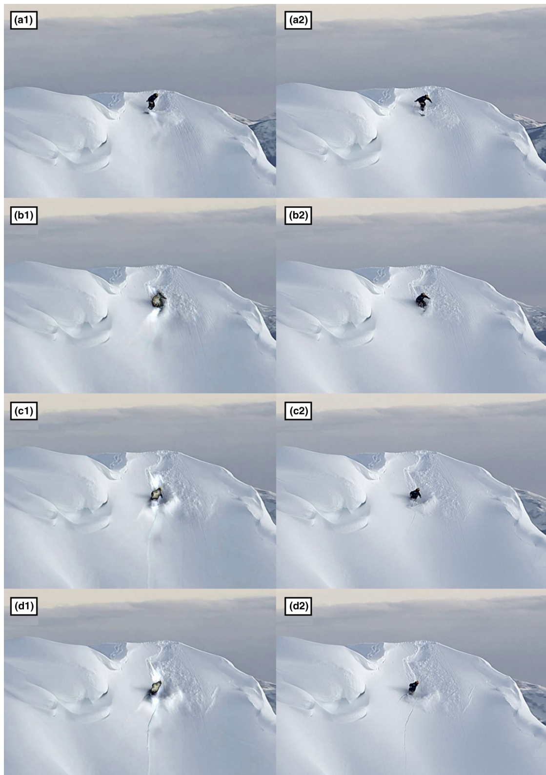
Figure 1. Comparison of enhanced (left) and original (right) frames extracted from a video of an avalanche from Alaska. We estimate that the crack in the weak layer was initiated at frame number 38. At frame number 37 (row A, 0.04 s. before crack initiation), snow surface movement from the snowboarder pushing the snow surface is visible up to 1.5 m downslope from the snowboarder. Frame number 47 (row B, 0.18 s. after crack initiation), snow surface movement is visible downslope from the snowboarder in the enhanced images (b1). Cracks on the snow surface below the snowboarder appear on frame 52 (c2, 0.28 s. after crack initiation), and snow surface movement becomes visible where the crown wall eventually develops to the left of the snowboarder (c1). In frame 56 (row D, 0.36 s. after crack initiation), the crown wall starts to appear on the snow surface in the original video (d2).
