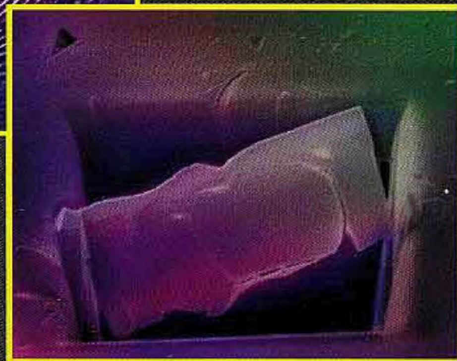
Image of a TEM sample of a lead-based ceramic prepared in an FEI Focussed Ion Beam (FIB) System (courtesy of Ed Gorzkowski, Lehigh University)
