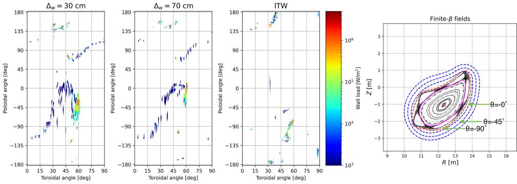
Figure 11: Power wall loads on the  $\theta\phi$ -plane for flat SOL profiles for wall with  $\Delta_w = 30$ ,  $\Delta_w = 70$ , and for the ITW. Only the first field period ( $0^\circ \leq \phi \leq 90^\circ$ ) is shown given the 4-field-period periodicity of wall loads in ASCOT5 simulations. Poincaré sections of Infinity Two at  $\phi = 60^\circ$  in the right panel show the approximate poloidal locations,  $\theta$ , where peak wall loads occur.
