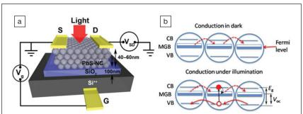
(a) A schematic of the optical field-effect transistor made from PbS nanocrystals (NCs) treated with ethanedithiol. (b) "Dark" conductance in NC films is mediated by midgap band states whereas photoconductance is dominated by photogenerated holes transported by quantum-confined NC states. MGB is mid-gap band, CB is conduction band, and VB is valence band. Reproduced with permission from *Nat. Commun.* (DOI: 10.1038/ncomms1492). © 2011 Macmillan Publishers Ltd.
