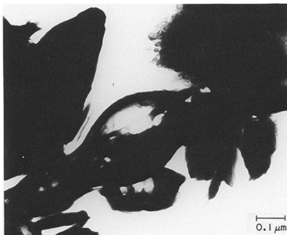
Figure 3. Kaolin particle flash-calcined in helium: edge view.
