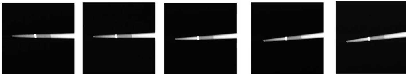
Figure 4. HAADF STEM images of the cylindrical specimen (-70, -35, 0, +35, +65)
