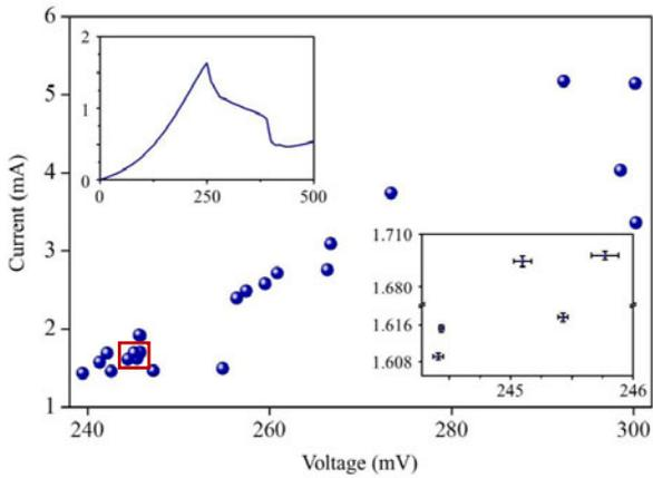
**Figure 2.** Peak voltage vs. current for 26 individual devices indicating the spread in results. The top-left inset shows typical measurement for a single device whilst the bottom-right inset displays the boxed region in finer detail.
