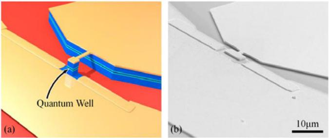
**Figure 1.** (a) An illustration of the resonant tunneling diode structure with a false z-scale to highlight the InGaAs/AlAs quantum well. (b) A scanning electron microscope image of a typical device.
