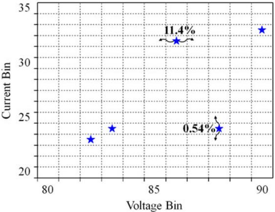
**Figure 3.** A subsection of the data from figure 2 replotted on scales with bins, to indicate how the quantum confinement physical unclonable function’s output could be digitized. The percentages indicate the probability of a measurement ‘hopping’ one bin along the two axes.
