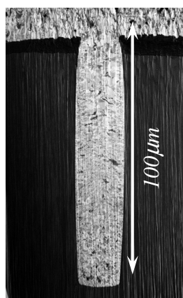
Fig.2. Deep Cross-sectional analysis of Through Silicon Via.
