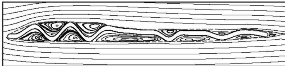
Figure 2. Time-averaged streamlines over a dragonfly's wing section (4) Reprinted from 'A computational study of the aerodynamic performance of a dragonfly wing section gliding flight' by A. Vargas, R. Mittal and H. Dong, 23/04/2008, Bioinspiration and Biomimetics , 3, (2), p 10.
