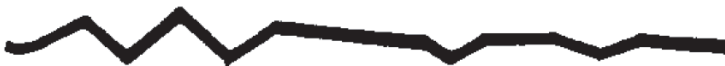
Figure 1. Wing-section of a dragonfly (3) . Reprinted from Aerodynamic characteristics of 'dragonfly wing sections compared with technical aerofoils' , by A.B. Kessel, 26/09/2000, Journal of Experimental Biology , 203 , (20), p 3126.
