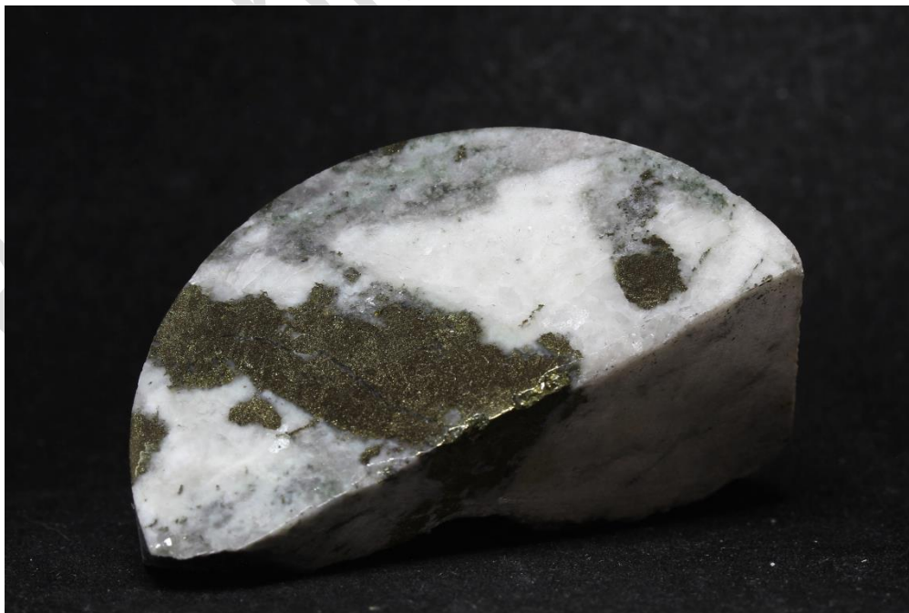
Figure 3. Fragment of drill core where tarutinoite was found. Dark areas are mainly composed of magnetite, chalcopyrite, pyrite and andradite. White is calcite. Size: 8 × 4 × 2 cm. Photo by Aleksey Podkorytov.
