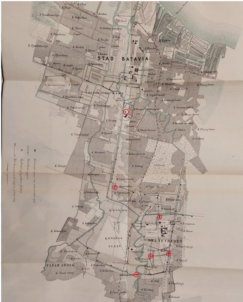
Figure 2. Map showing Batavia’s artesian wells (circled in red) and hydrants and fountains (round black dots), 1879. From the Jaarboek van het mijnwezen in Nederlandsch Indië ( Yearbook of the mining industry in the Netherlands Indies ), 8, no. 1 (1879). Red annotations by present author.
