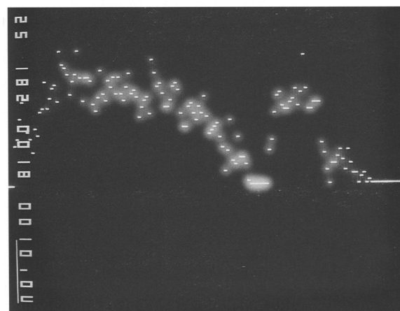
Figure 4. EMPA of an Fe oxide aggregate for a sample taken immediately after coprecipitate formation by rapid titration ( t = 0 d). a) Fe oxide aggregate, b) line scan of Cu and c) line scan of Zn. Line scans were taken along the horizontal line on (a). Horizontal lines on (b) and (c) are baseline levels resulting from cracks in the aggregate after application of 100 nA current.
