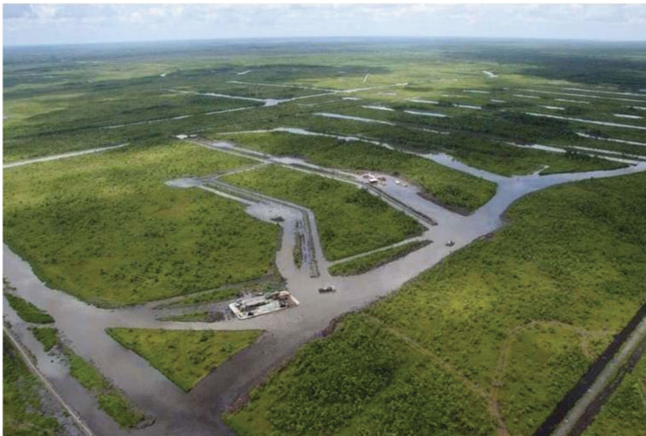
Fig. 14. A developed swamp area in the field with the individual well locations connected by water trails.
