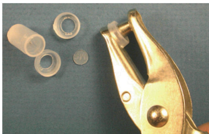
Figure 2. Chamber manufacture. (a) Preparing the capsules. Half the capsules are used for chambers and top caps; half, for bottom caps. Stainless steel disks are tamped into punched caps with a 11/32" drift. (b) Modified 1/4" hole punch is centered in top of each cap, die below.
