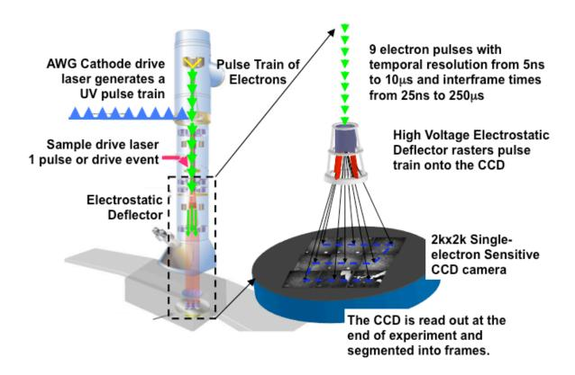
FIG 1. Schematic of the Movie Mode technology that enables single-pump/multi-probe operation and true, in-situ microscopy capabilities in the DTEM in which multi-frame movies of ultrafast material dynamics can be acquired.
