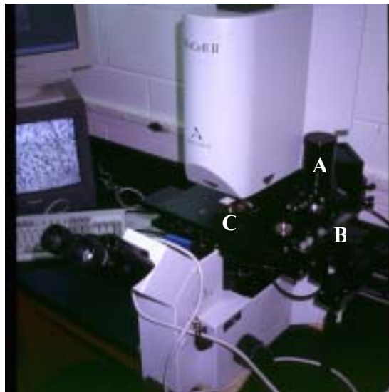
FIG. 2. View of LCM laser and microscope stage with mechanical arm (A) used to move small caps with transfer film (B) over an uncoverslipped tissue section on a glass slide (C).
