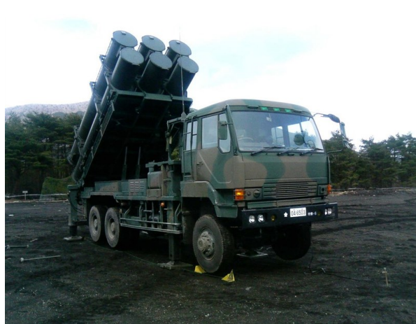
Truck carrying Type 88 missiles. Also known as SSM-1 or Shibasuta, this missile was developed by Mitsubishi Heavy Industries from the Air SDF Type 80 (ASM-1) air-to-surface anti-ship missile. 28
