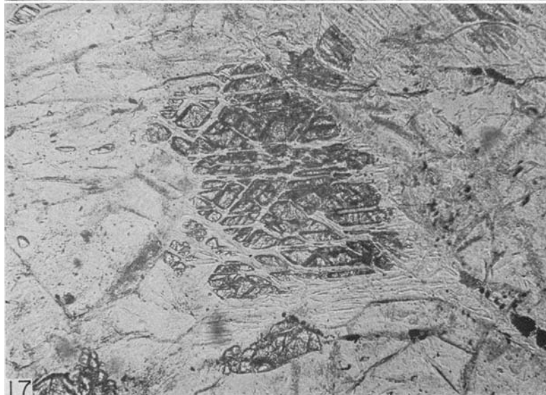
Fig. 16. Photomicrograph of a thin section of sample 487-44-28, showing relict olivine ( \text{Mg}_{1.82}\text{Fe}_{0.18}\text{SiO}_4 ) in serpentine. Polarized light. Magnification = 130\times .
