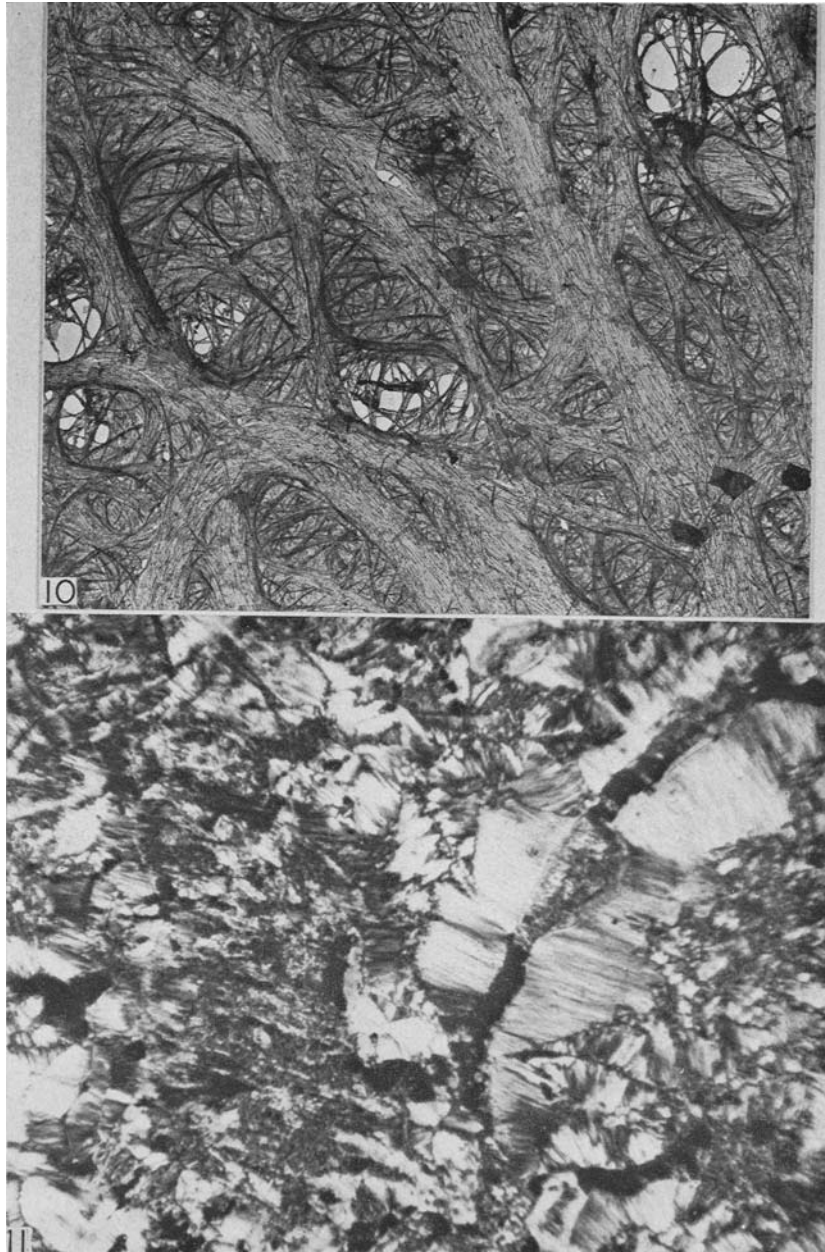
Fig. 10. Electron micrograph of a replica of chrysotile from the leathery sheets from the Coalinga asbestos deposit. Magnification = 5000 \times .
