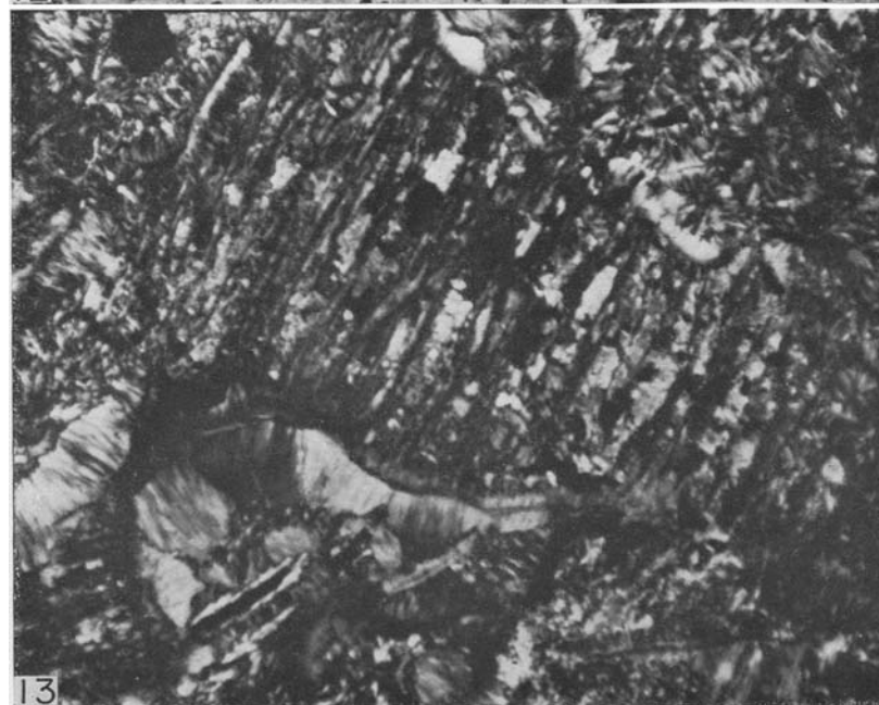
Fig. 12. Photomicrograph of a thin section of sample 487-44-9 showing serpentine (white-gray) with characteristic "mesh" structure and magnetite (black). Polarized light. Magnification = 50 \times . Fig. 13. Photomicrograph of a thin section of sample 487-44-6 showing serpentine, brucite and magnetite. Crossed nicols. Magnification = 50 \times .
