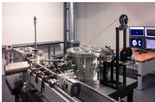
Figure 1. The SiriusXT compact Soft X-ray microscope, with an overall footprint of 3m x 2m.
