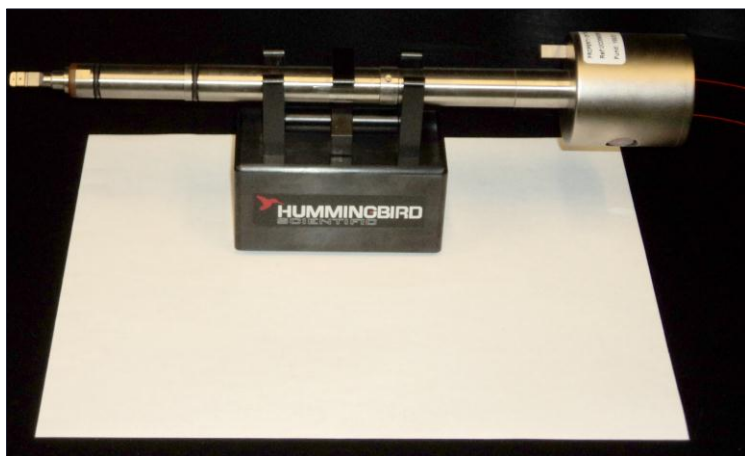
FIG. 1. Hummingbird Scientific fluid stage holder equipped with inlet and outlet lines for microfluidic pumping. The window region well holds two 2.6 \times 2.6 \times 0.3 \mu\text{m} windows, composed of electron transparent SiN thin film membrane supported by Si substrate. 50 nm Au spacers were deposited at the window corners.
