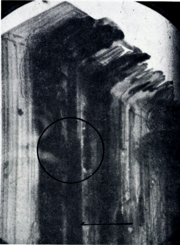
Fig. 5. X-ray topogram of crystal with high dislocation density. Dielectric relaxation of the circled portion is shown in Figure 6. Length of diffraction vector (arrow) is 1 mm.
