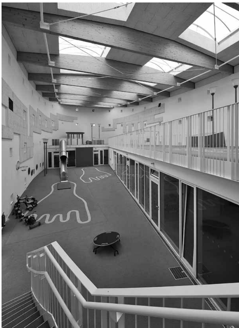
16 View from the top floor east end, showing the upper volume of the former church and the daylight flooding in through the roof. Climatically it serves as a buffer space.
