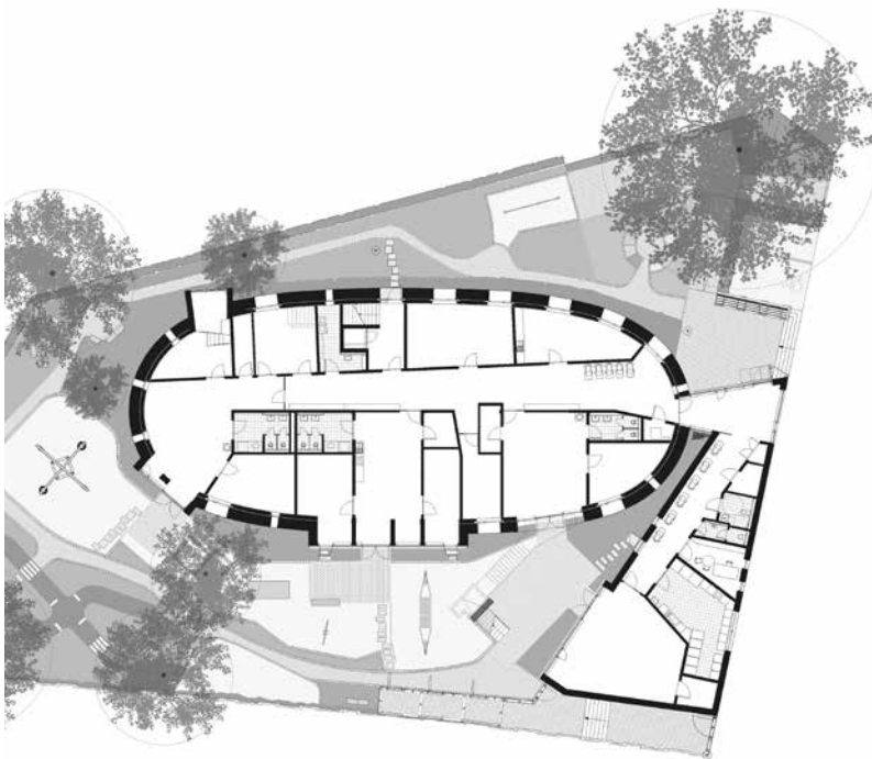
12 Conversion of St Sebastian, ground floor plan. Entrance is from the east, playground to south and west. The new wedge-shaped building bottom right includes kitchen and dining room.
