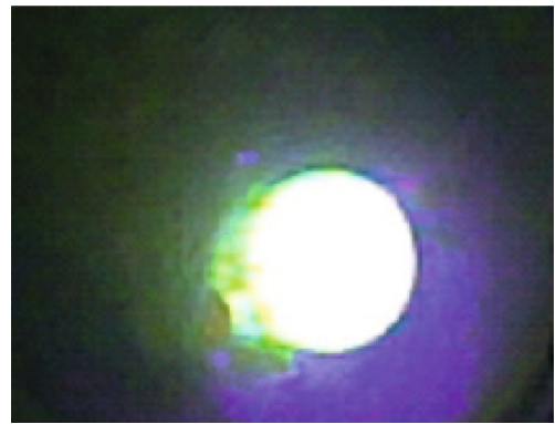
Fig. 4. (Color online) (a) Tristimulus coordinates of CdS nanoparticle (0.37, 0.34) on the CIE 1931 chromaticity diagram. (b) A photograph of white light generation from illuminated CdS/PMMA composite film by UVGaN-LED.
