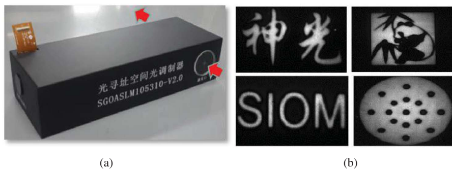
Figure 29. (a) Optical addressing liquid crystal spatial light modulator physical map. (b) Near-field spatial intensity distribution control demonstration.
