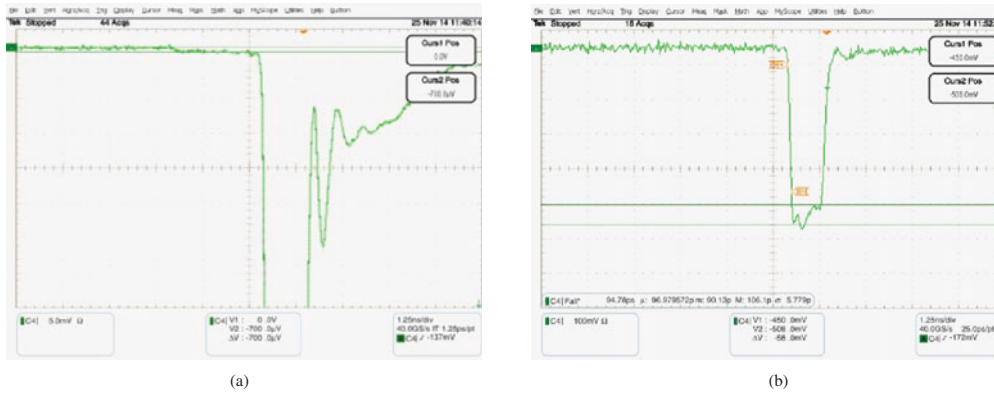
Figure 15. The high contrast temporal waveform (600 : 1). (a) Low amplitude pedestal; (b) high amplitude step.
