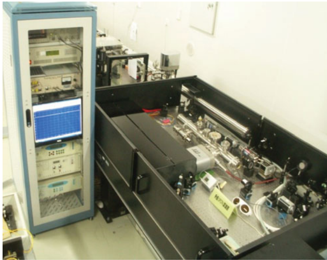
Figure 45. The OPCPA pump source includes: Nd:YAG regenerative amplifier, beam expander, soft-edge iris, spatial filter, three-stage Nd:YAG rod amplifier and frequency multiplier.
