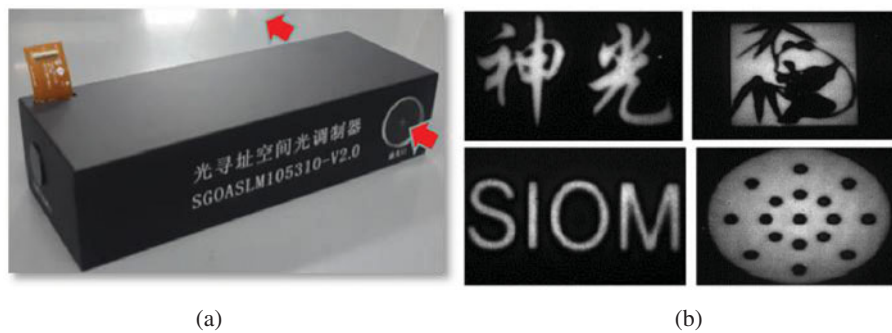
Figure 29. (a) Optical addressing liquid crystal spatial light modulator physical map. (b) Near-field spatial intensity distribution control demonstration.
