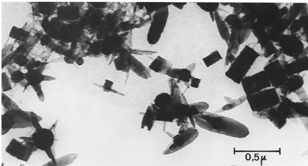
Figure 5. Transmission electron micrograph of hematite (70%) and goethite (30%) formed in the presence of 10^{-4} M glucose (pH 11.1, 70°C).
