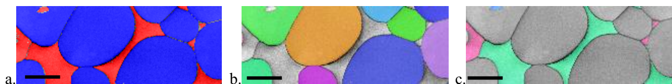
Figure 1. Example portions of EBSD maps from a W-hardened alloy. (a) Phase, with blue = W, red = Ni; Orientation maps for (b) W and (c) Ni, based on a surface normal-projected IPF. Scale bar = 10 \mu m.
