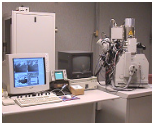
FIG. 1. The FEI Strata™ DB 235 at the Princeton Materials Institute incorporates both a focused gallium ion beam as well as a scanning electron microscope. The SEM column is above the chamber while the ion beam column is attached towards the side at 52° angle. The precision provided by the exactness of the ion beam machining and the high resolution imaging of the SEM provide the ability to prepare various samples and to perform in situ fabrication with observation.
