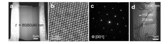
**Figure 1.** (a) FIB sample of Fe3Sn2 with varied thickness of 40 nm, 60 nm, and 80 nm. (b) HRTEM image and (c) SAED pattern of Fe3Sn2 sample. (d) Lorentz TEM image of 40 nm thick Fe3Sn2 showing the stripe domain structures with different domain widths.
