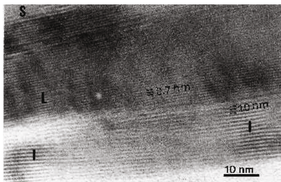
Figure 7. HRTEM images of 0.7 and 1.0 nm intergrowths. I = illite, L = ferroan lizardite (see discussion for explanation), and S = smectite.
