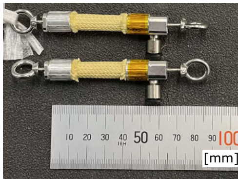
Figure 6. Small PAMs for force estimation.
