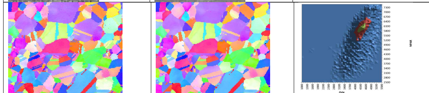
Figure 2. IPF maps of nickel show (a) high quality maps, (b) NPAR processing map which reduces the noise associated with boundary edges but also “removes” very thin twins and grains, and (c) a plot of the pixel IQ values before and after NPAR processing.
