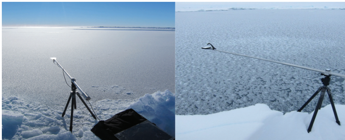
Fig. 2. Photographs showing ASD spectral radiometer. The ASD is contained in the sled (seen in left photograph) and is connected to a cosine collector on the far end of the metal rod by a fiber-optic cable. The rod contains a counterweight on the end closest to the ASD, and a tripod is used to steady the rod. The rod can be rotated to position the diffuser plate downward towards the ice surface and upwards towards the sky. The ASD is used here to measure the albedo of a dense frost-flower field covering nilas (left, 4 October 2012) and sparse frost-flower field covering nilas (right, 28 September 2012).
