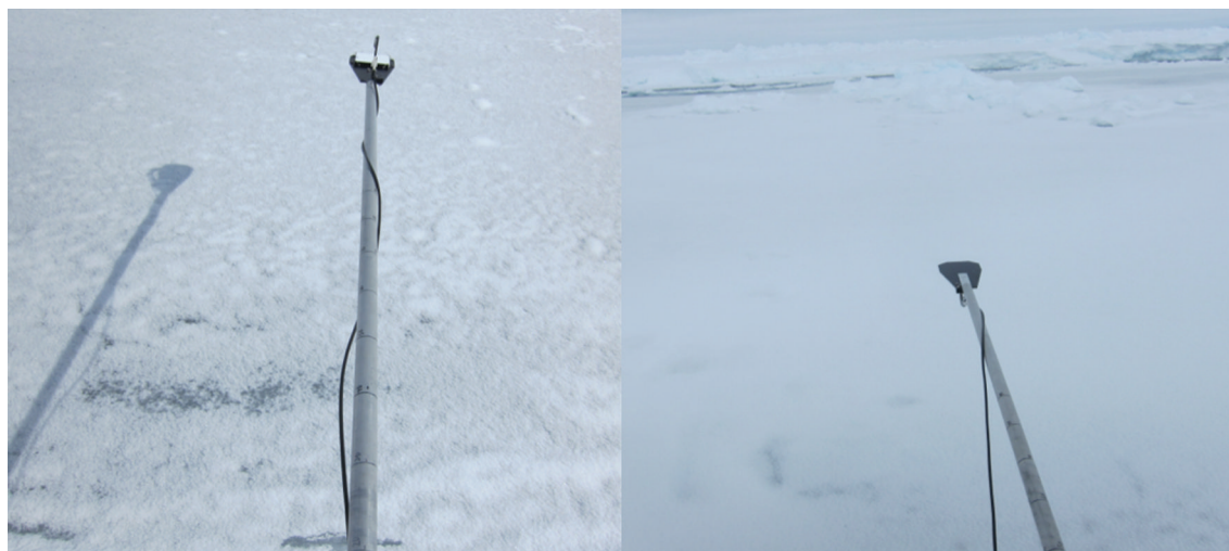
Fig. 10. Photographs of three-layer surface types taken on 2 November 2012. Left: 0.5 cm of snow covering 10 cm of slush covering 16 cm of ice. Right: 2 cm of snow covering 3 cm of slush covering 12 cm of ice. Albedos for these scenes are shown in Figure 11.
