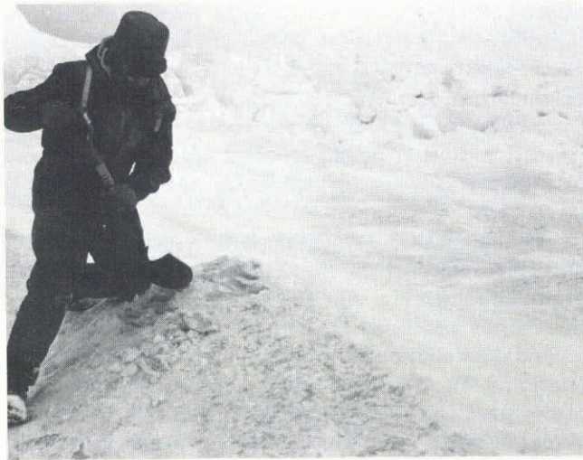
Fig. 7. Dirty, hard snow chipped from a 2 m 2 area on the surface of this old drift at station 34 contained 400 ml of wet sediment.
