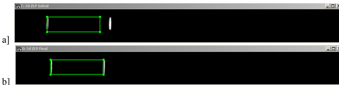
Fig. 3. Dispersion Height and Focus tuning. Fig. 3a] shows the initial, untuned state. The green annotation reflects the target height and dispersion for the 2 zlp peaks. Fig. 3b] demonstrates the result after auto-tuning.
