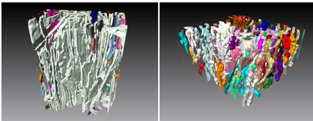
Figure 1. Reconstruction from FIB/SEM tomography of the eutectic silicon in an unmodified Al-7wt%Si alloy (left), approx. 70 \times 100 \times 40 \mu\text{m}^3 and in a Sr-modified Al-7wt%Si alloy (right), approx. 37 \times 17 \times 35 \mu\text{m}^3 .
