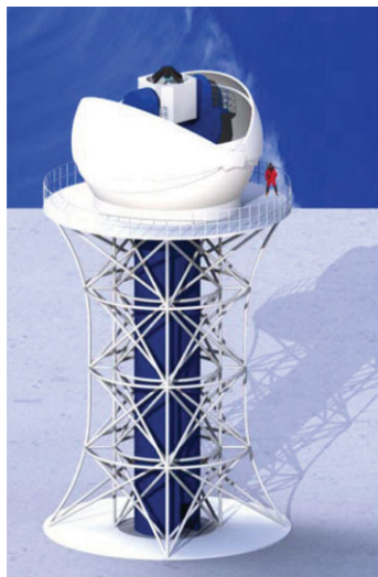
Figure 2. Model of KDUST with compact structure, open dome and 15 m tower.
