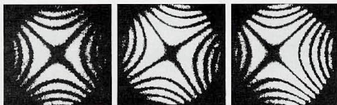
Figure 2: The interference pattern from a quartz crystal. The cross in the middle figure shows the direction of the analyzer and polarizer. The left interference figure shows the crystal with its optic axis normal to the optic axis of the microscope. The middle interference figure shows the crystal with its optic axis rotated in a plane normal to the optic axis of the microscope and the right interference figure shows the crystal with its optic axis tilted.
