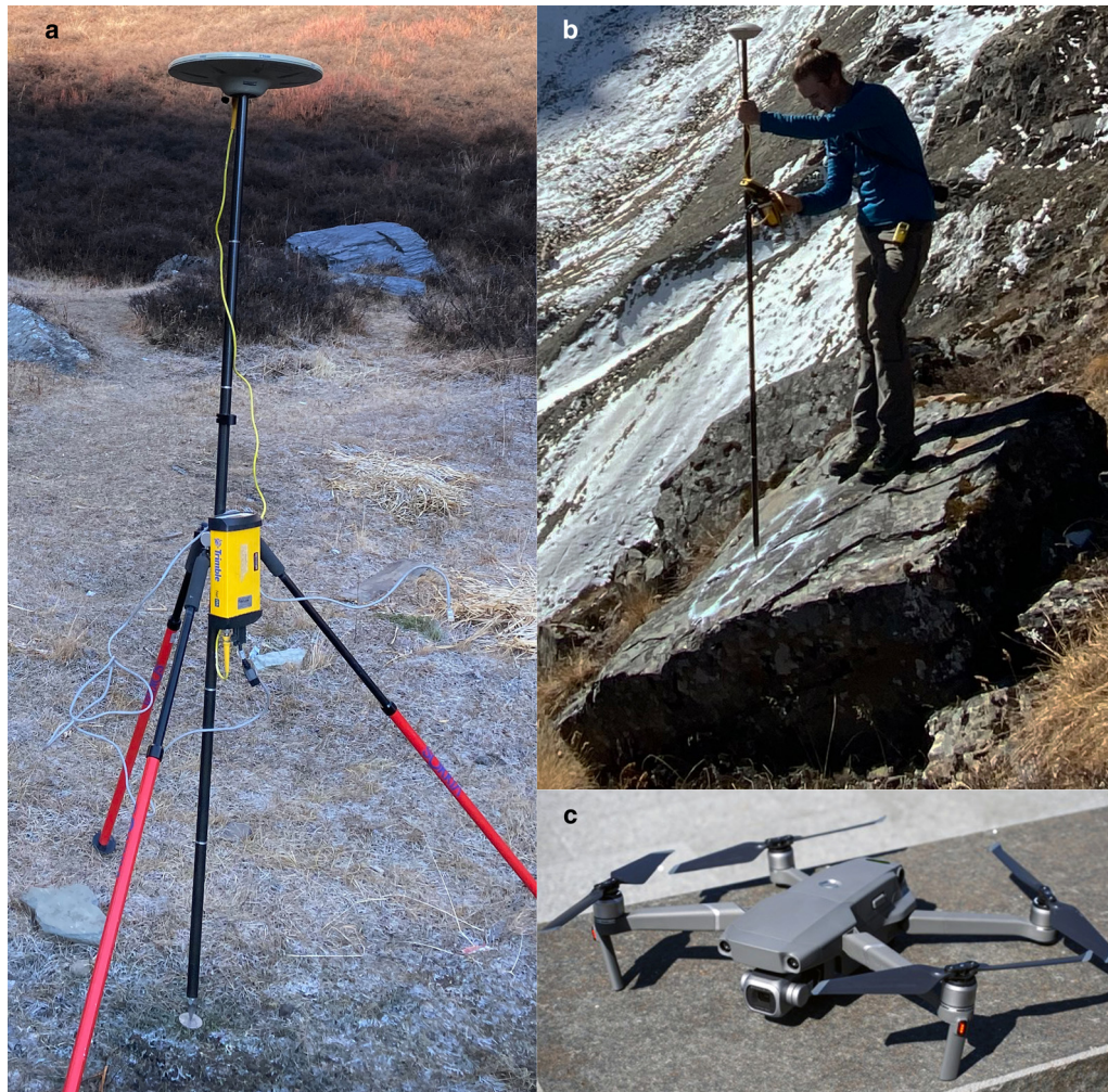
Fig. 3. (a) A differential GNSS base station (location shown in Fig. 2), (b) the GNSS rover collecting data over a marked GCP and (c) the utilized quadcopter UAS.
