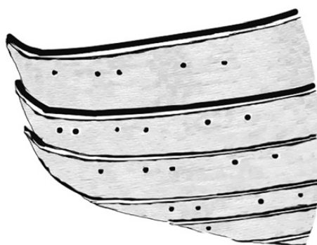
Figure 27 Overlapping, clinker-built hull construction.
