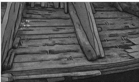
Figure 14 Quanzhou Ship Hull Planking, Fastenings, Ribs, and Bulkhead, Quanzhou Maritime Museum
