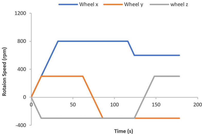
Figure 3. Alsat-1B wheel rotational speed profile.
