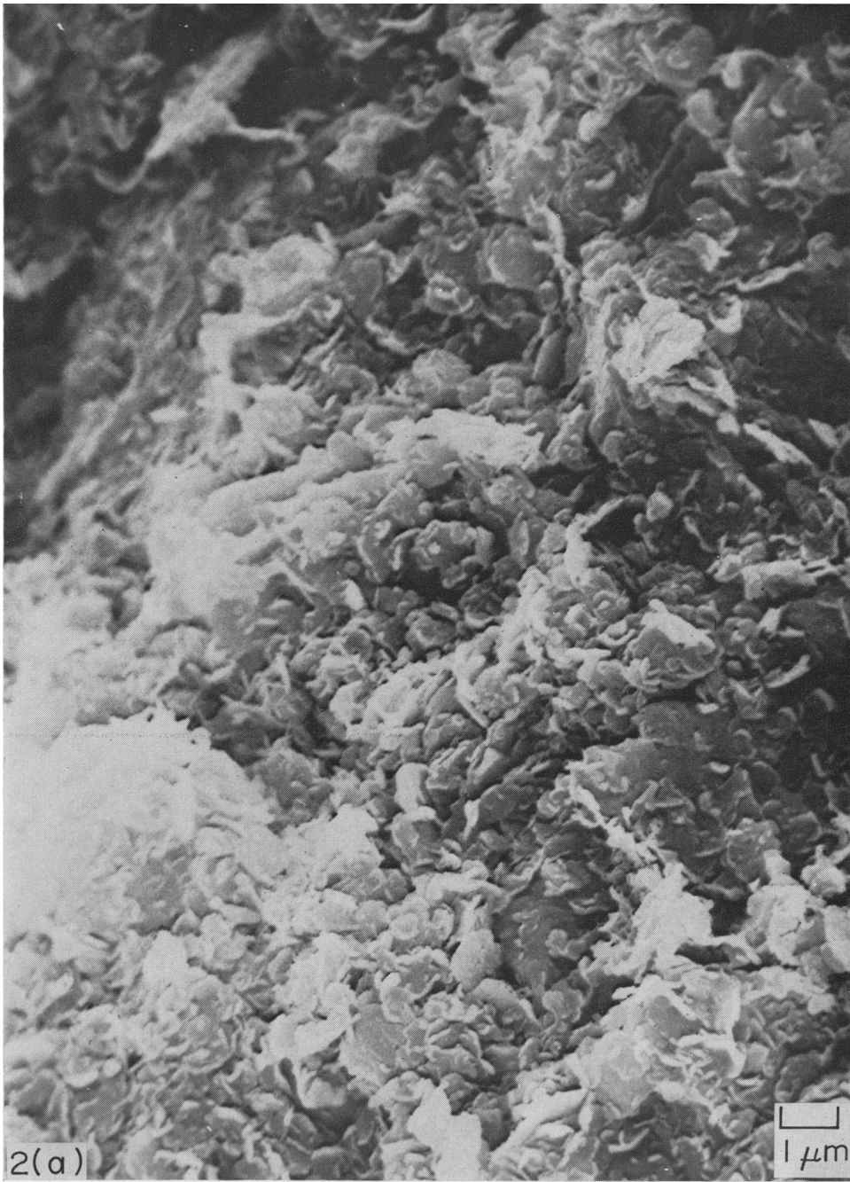
Fig. 2. Critical-point dried, electrostatically cleaned submarine sediment (Mississippi Delta); (a) general view, (b) detail of EE, EF structure (rosette).
