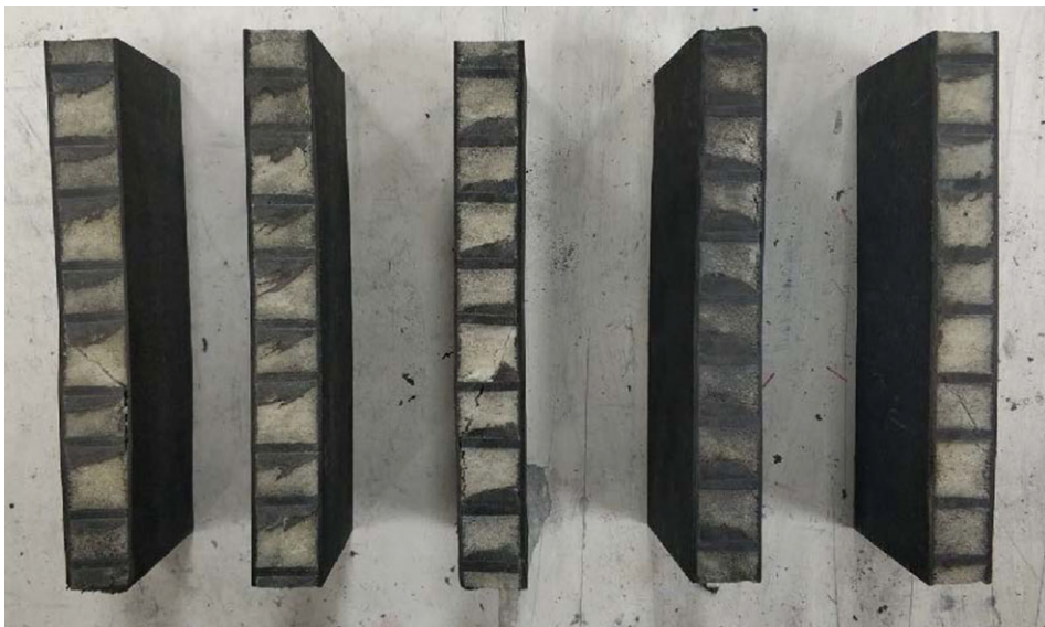
Figure 12. Failures in polyurethane foam-filled specimens in the three-point bending test.
